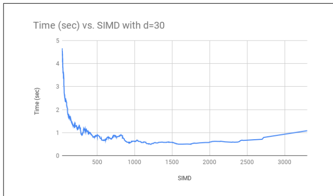
Figure 9: Run-time of LHE operations ( y -axis in seconds) on d = 30 and increasing number of slots sl ( x -axis).
