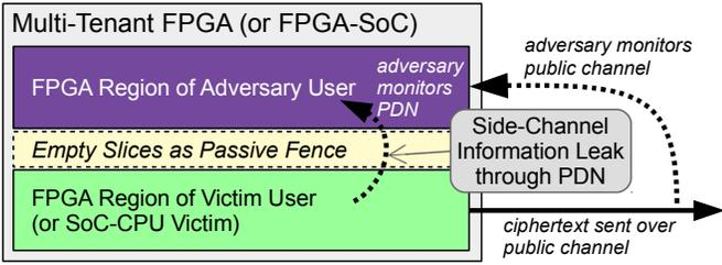
Fig. 1: Adversary model for a multi-tenant FPGA or FPGA with shared SoC Logic, such as ASIC-logic CPUs. Based on the models previously shown in [33], [38].
