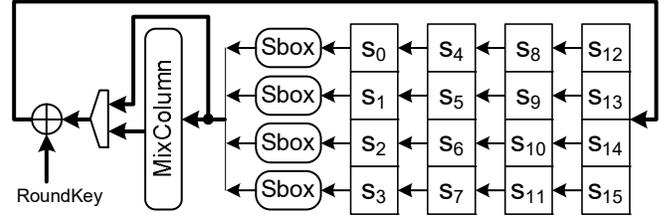
Fig. 8: Schematic of the used AES encryption core design as shown in [33]
