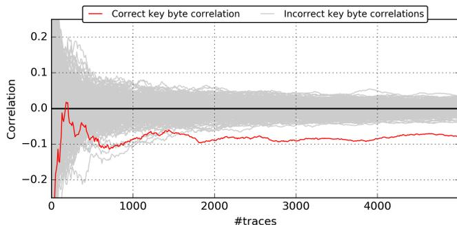
Fig. 10: Baseline results for CPA on AES without any countermeasure. The correlation for the correct key is marked red and the attack is successful after about 1800 traces.
