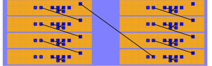
Fig. 9: Partial sensor carry-chain on the ECP5 as displayed in the Floorplan View of the Lattice Diamond design software; Each block contains a 2-bit carry element and the connection between those elements enforces adjacent placement as a fast carry chain on the ECP5
