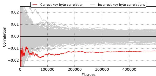
Fig. 11: Results for CPA on AES with an arbitrarily placed active fence, activated based on a PRNG output. The correlation for the correct key is marked red and the attack is successful after about 80k traces.
