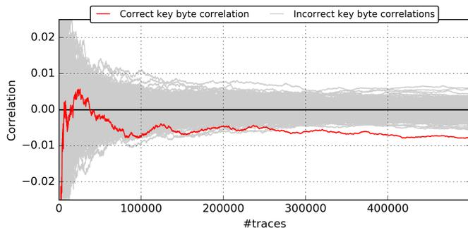
Fig. 13: Results for CPA on AES with a sensor-based active fence, that is placed row-by-row. The correlation for the correct key is marked red and the attack is successful after about 300k traces.
