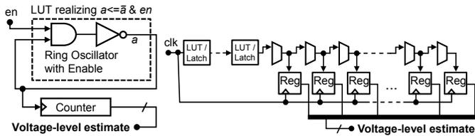
Fig. 2: Two types of voltage side-channel sensors in an FPGA as shown in [18]. Left: RO counter, right: tapped delay line.
