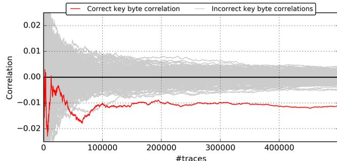
Fig. 12: Results for CPA on AES with an active fence, that is placed row-by-row and activated based on a PRNG output. The correlation for the correct key is marked red and the attack is successful after about 120k traces.
