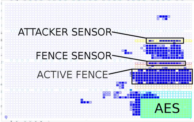
Fig. 7: The complete layout of the design on the ECP5 FPGA as seen in the Lattice Diamond Floorplan Viewer
