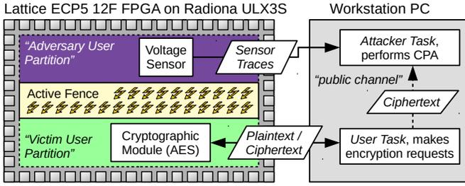
Fig. 6: Experimental setup overview showing the Lattice ECP5 FPGA connected to a workstation PC. The AES module is used to encrypt messages, while an attacker can use the ciphertexts together with sensor traces to perform CPA.
