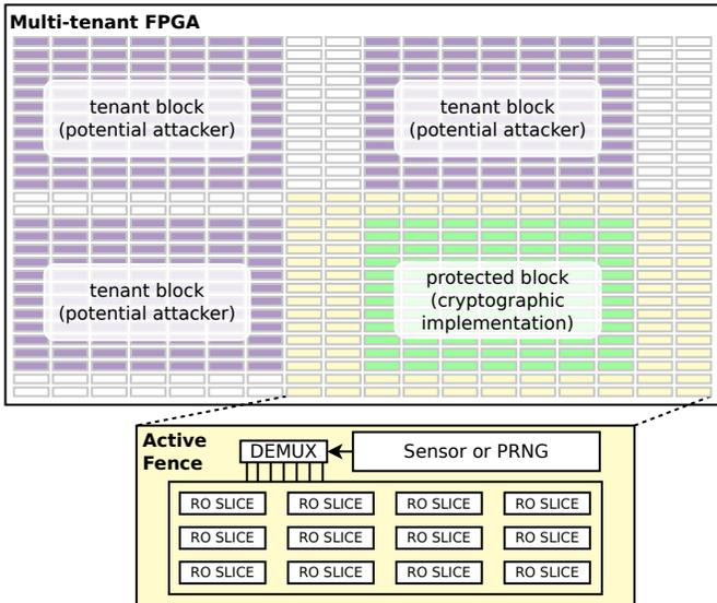
Fig. 3: Overview of the active fence as a protective countermeasure between a design, which is used in a security-related application, and other users on a multi-tenant FPGA. A specific amount of ROs is activated dependent on the value of a sensor or a Pseudo-Random Number Generator (PRNG).
