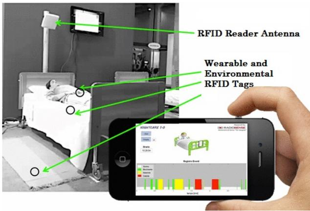
Fig. 2: The night-care system, an ambient RFID-based intelligence system for different health-care purposes in the IoT [10].
