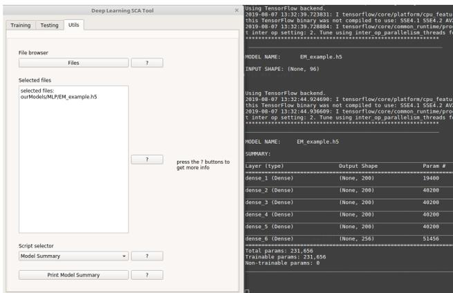
Figure 7. Results of running scripts for input shape and model summary
