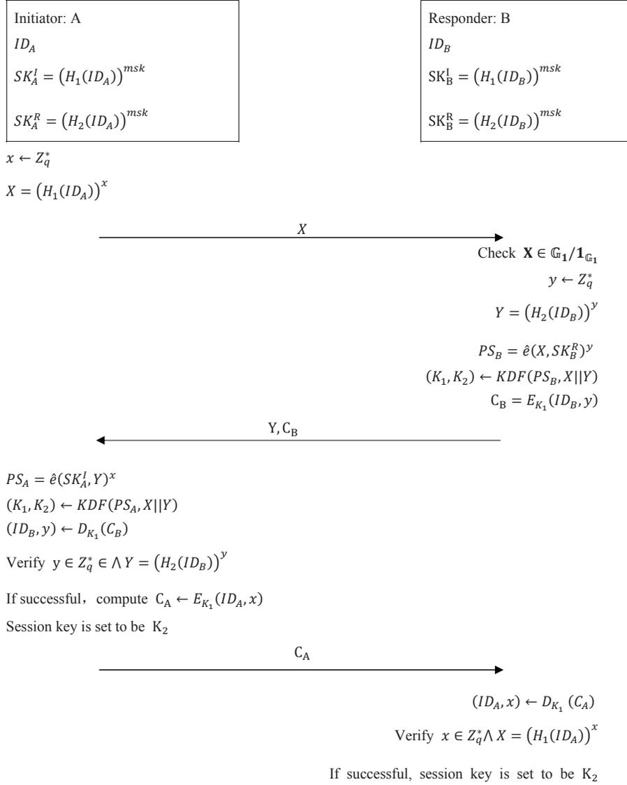
**Fig. 5.** Construction of IB-CAKE with Type-III Bilinear Mapping
