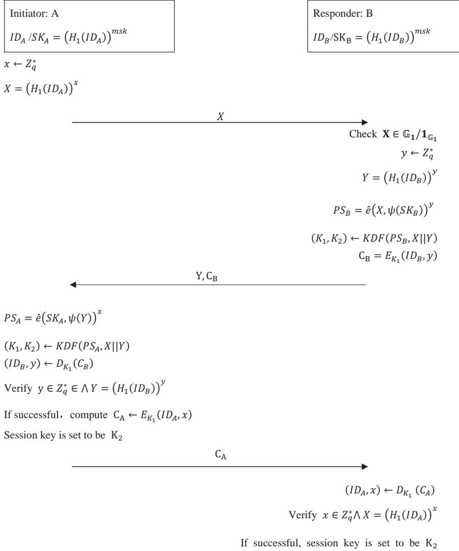
**Fig. 4.** Construction of IB-CAKE with Type-II Bilinear Mapping
