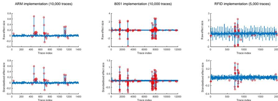
**Fig. 2.** Difference of means (top) and standardised equivalent (bottom) associated with the first bit of the first S-box of two software AES implementations and the first bit of the second S-box of one hardware implementation. Red circles denote points where a distance-of-means attack achieves stable key recovery.
