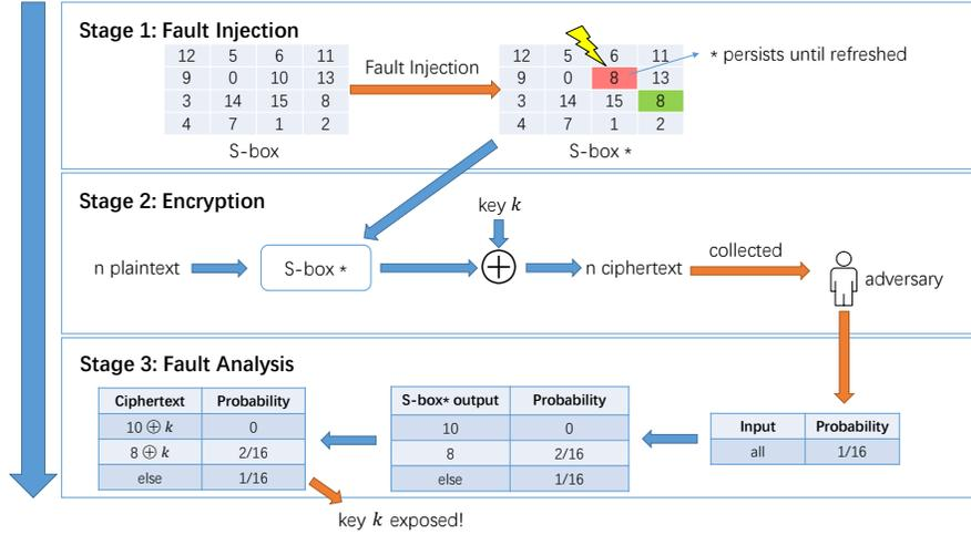
Fig. 1. Overview of Persistent Fault Attack.
