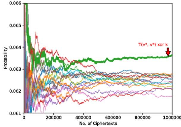
Fig. 4. Key Extraction with  $t_{max}$  strategy on Software TI [13].
