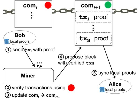
Figure 1: EDRAW architecture. Transactions include proofs. Miners verify transactions using the block commitment  $com_t$  stored at the last block  $t$ , an updated version of which is included in the next block  $t + 1$ . Clients synchronize their local proofs after the new block is produced.
