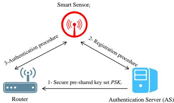
**Fig. 1.** System model of M2M technology employed in IIoT
