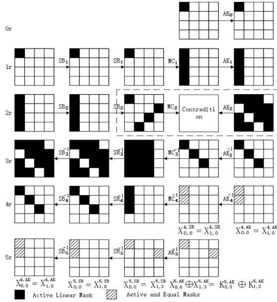
Fig. 4: ZC Linear Hull of 5-Round AES [12].
