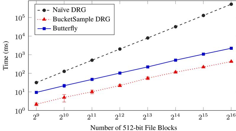
**Figure 5:** Fast operation overhead for different layer types and sizes. Naïve DRG run time grows quadratically with the graph size, while the others grow roughly linearly.
