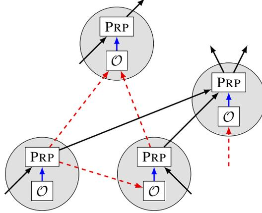
**Figure 2:** The high level structure of an encoding based on a DAG. Solid black edges are data edges, dashed red edges are key edges, and blue arrows from  $\mathcal{O}$  to PRP show the use of derived keys.
