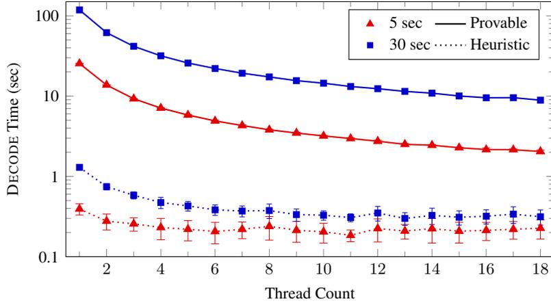
**Figure 7:** DECODE time for a 256 KiB file for both 5 and 30-sec security bounds run with multiple threads on an Amazon EC2 c5.18xlarge. Solid lines use a provably-secure naïve DRG and script. Dotted lines use a heuristic DRG and Sloth.
