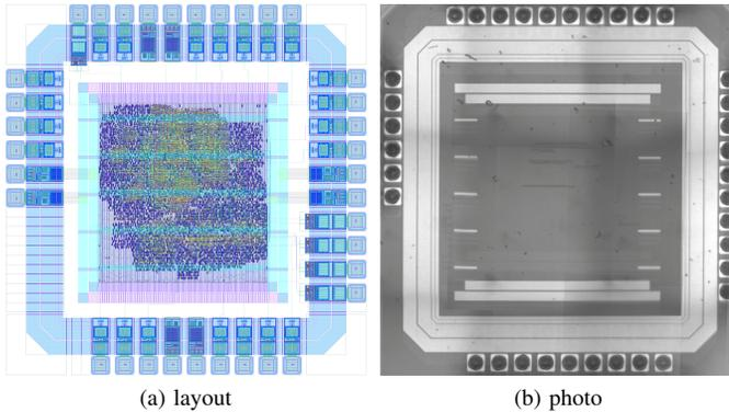
Fig. 6: ASIC prototype with 6 cores in 150 nm CMOS [27].
