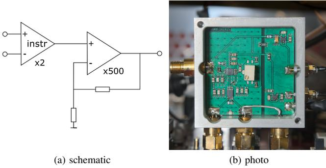
Fig. 1: Low-noise DC amplifier for static power measurements.
