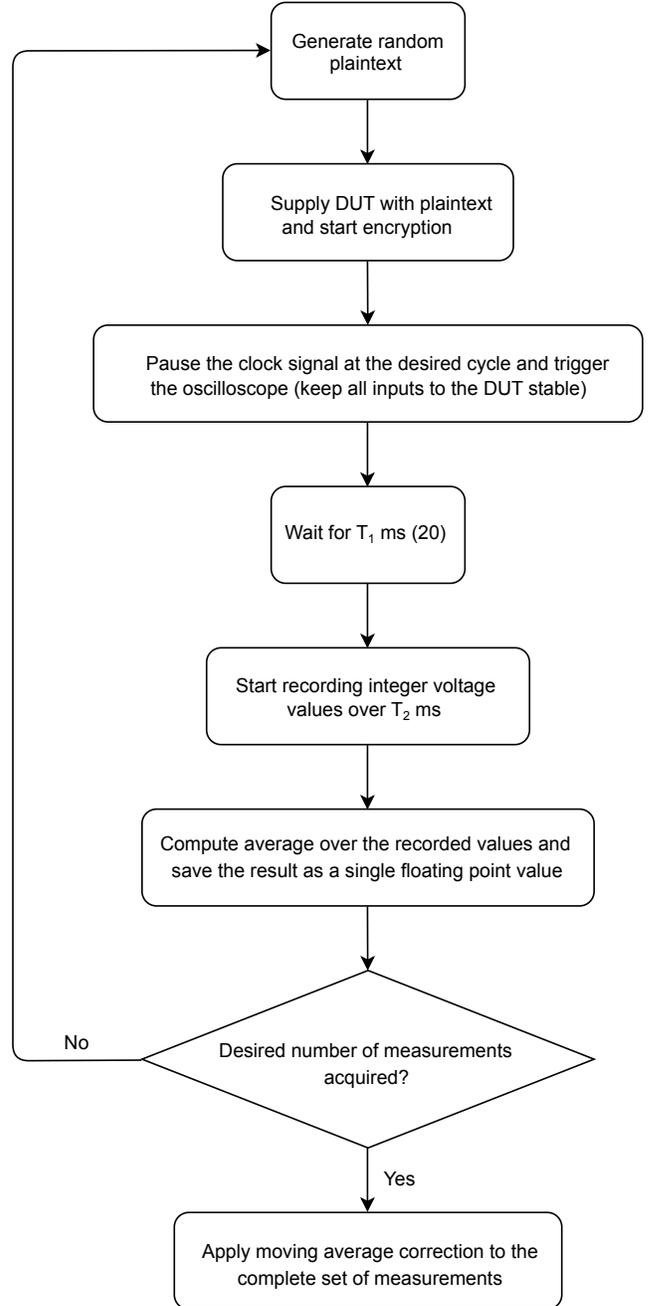
Fig. 9: Flowchart describing the measurement procedure. simple flowchart.
