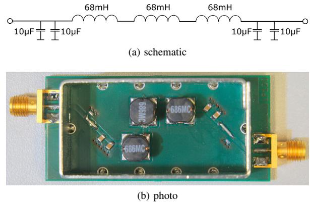
Fig. 2: Third-order (Butterworth Pi) LC low pass filter with cutoff-frequency of  $\sim 100 \text{ Hz}$ .
