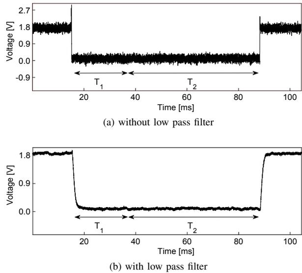
Fig. 3: Exemplary depiction of two measurements, one with and one without low-pass filter, for a measurement interval of  $50 \text{ ms}$ . Time period  $T_1$  (here  $20 \text{ ms}$ ) corresponds to the interval that is ignored due to the memory effect. Time period  $T_2$  (here  $50 \text{ ms}$ ) corresponds to the measurement interval. All values that are measured in  $T_2$  are averaged to a singular static power value.
