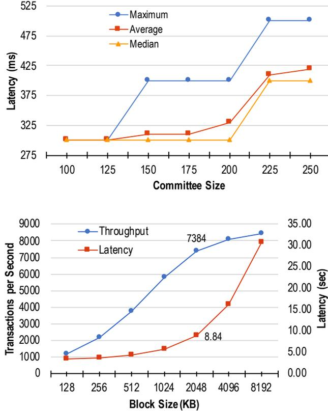
Figure 4: Latency of gossiping an 80-byte message for different committee sizes (left); Impact of block size on throughput and latency (right)
