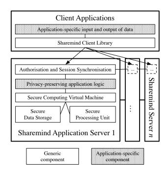
Fig. 4. Simplified architecture of the Sharemind platform  $% \mathcal{F}_{\mathrm{s}}^{(1)}(\mathcal{F}_{\mathrm{s}})$
