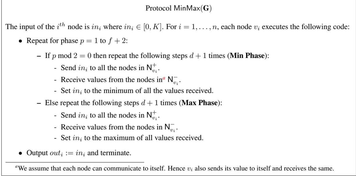
Figure 1: Multi-valued crash-tolerant consensus based on min-max strategy
