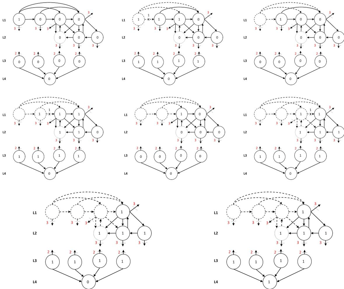
Figure 10: The graph showing the impossibility of achieving consensus within  $2f + 1$  phases for  $f = 3$  and  $d = 2$ . The figures from left to right show the value of nodes in each graph at the end of the first, second, third, fourth, fifth, sixth, seventh and eighth phase respectively.
