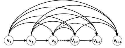
Figure 2: The family of graphs in which it is impossible to achieve consensus in  $f + 1$  phases.
