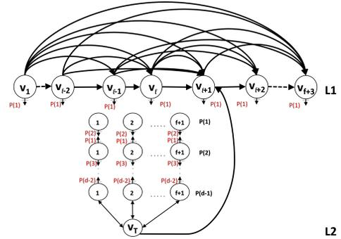
Figure 5: The family of graphs in which it is impossible to achieve consensus in  $f + 2$  phases with each round having at least  $d$  rounds and with total  $(f + 2)(d + 1) - 3$  rounds.
