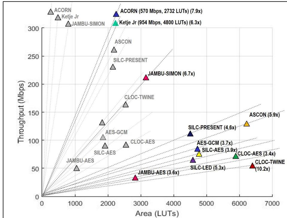
Fig. 20. Throughput, area (in LUTs), and throughput-to-area (TP/A) ratios of unprotected and protected authenticated ciphers. Unprotected versions are shown in gray triangles, while protected versions are depicted with darker triangles. The relative increase in TP/A ratio is shown next to protected versions.
