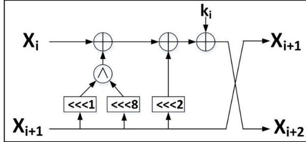
Fig. 9. One round of SIMON 96/96 primitive used in JAMBU-SIMON. All bus widths are 48 bits.
