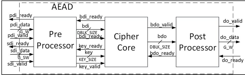
Fig. 3. External interface of the authenticated cipher module (AEAD), compliant with the CAESAR Hardware API [5, 6], and the internal top-level block diagram of AEAD supported by the Development Package [7].
