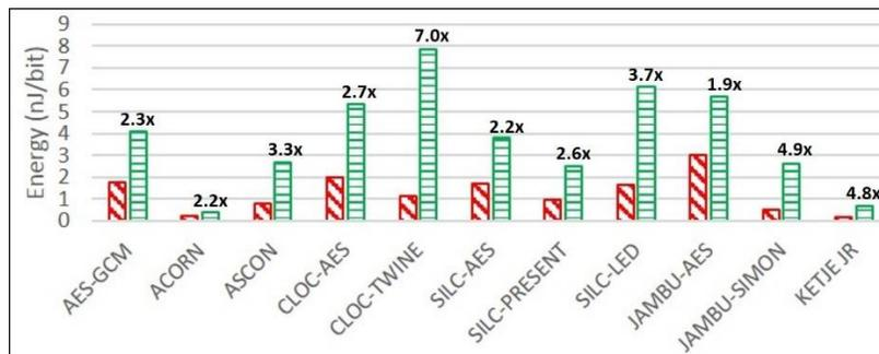
Fig. 22. Energy-per-bit of unprotected (using diagonal lines) and protected (using horizontal lines) cipher versions, measured as described in subsections 3.2 and 5.6. The relative increase is shown above protected versions.
