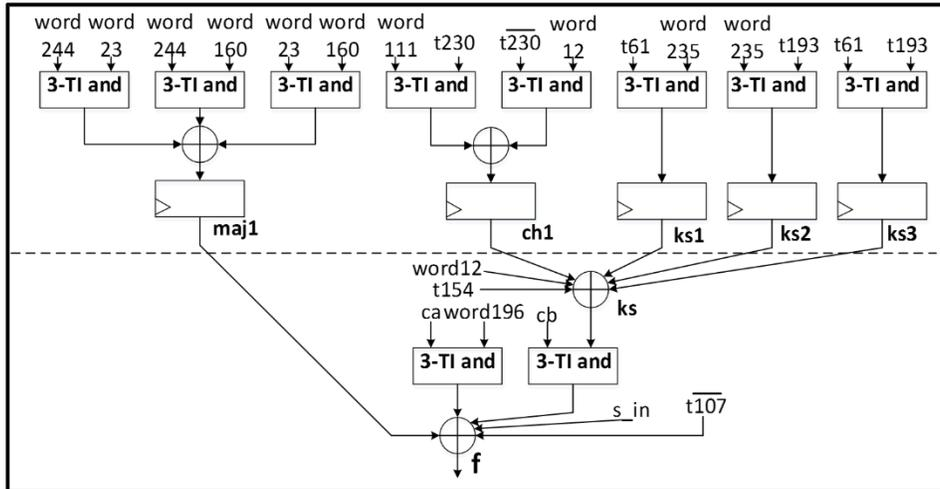
Fig. 5. Simplified ACORN two-cycle state update. Dashed line indicates boundary between clock cycles. All signals and buses represent two TI-shares. Signals are defined in source code [16], and derived from [9]. All bus widths are 8 bits.
