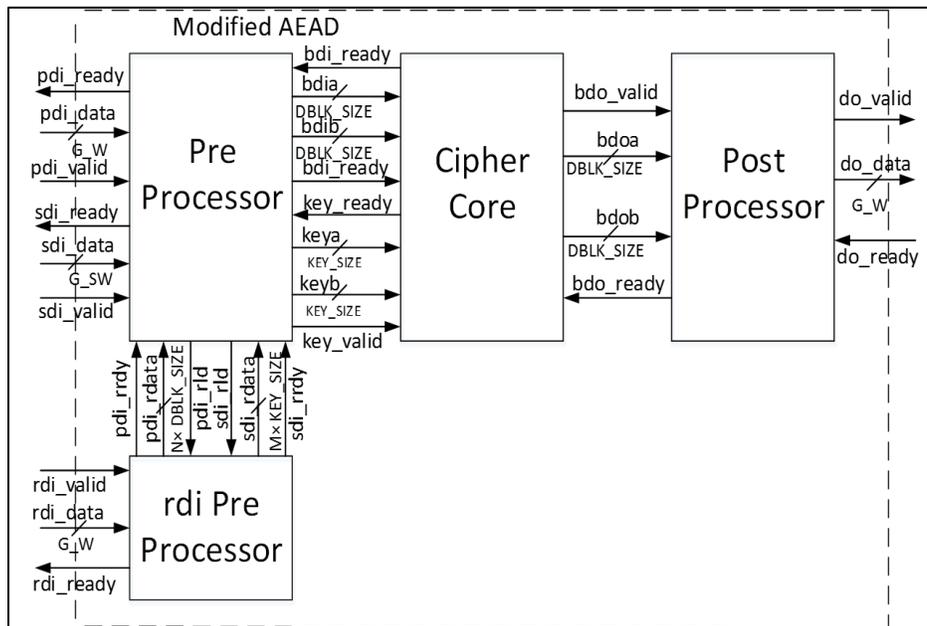
Fig. 16. External interface of the modified authenticated cipher module (Modified AEAD), and the internal top-level block diagram of Modified AEAD, augmented with rdi PreProcessor
