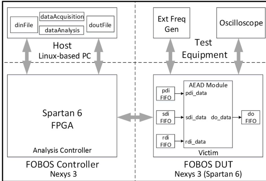
Fig. 4. FOBOS architecture modified for t-test leakage detection on authenticated ciphers
