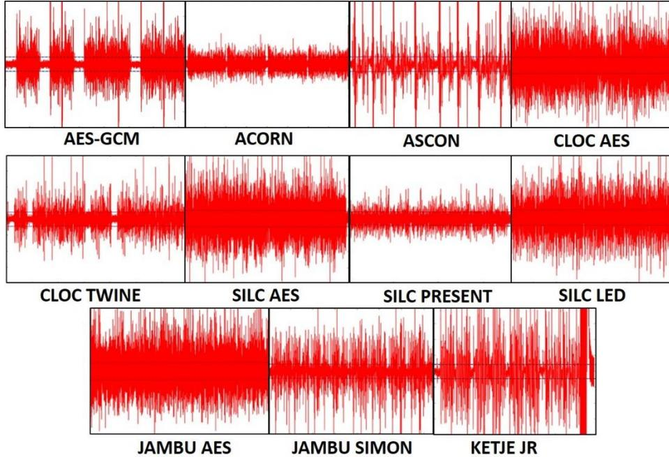
Fig. 13. Results of t-test on unprotected ciphers. Time domain (samples) are on the x-axis, t-values are on the y-axis. Horizontal lines denote  $t = \pm 4.5$ .
