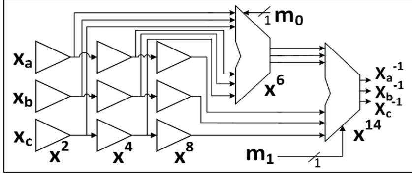
Fig. 11 3-share TI  $GF(2^4)$  inverter used in TWINE.  $x^2, x^4, x^8$  (produced by squares), and  $x^6$  (where  $x^6 = x^2 \cdot x^4$ ) are intermediate products;  $x^{14}$  (where  $x^{14} = x^6 \cdot x^8$ ) is final product; All bus widths are 4 bits, except for random bits  $m_0$  and  $m_1$ , which are single bits. Adapted from [22].
