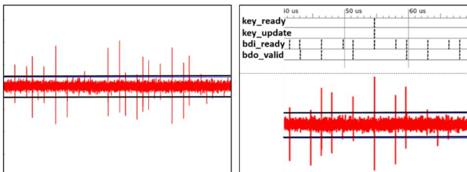
Fig. 14(a) (left) T-test result for protected version of AES-JAMBU CipherCore; 14(b) (right) Time-domain alignment of leakage spikes with key I/O signal events in Xilinx iSim simulation of the same cipher.
