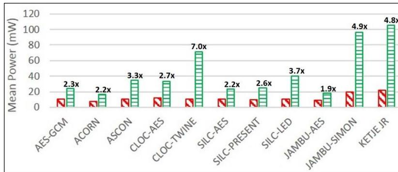
Fig. 21. Mean power of unprotected (using diagonal lines) and protected (using horizontal lines) cipher versions, measured as described in subsections 3.2 and 5.6. The relative increase is shown above protected versions.
