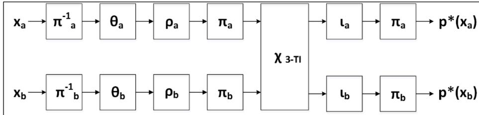
Fig. 12 Hybrid 2-/3-share TI-protected Keccak- $p^*$  transformation, used in Ketje Jr.
