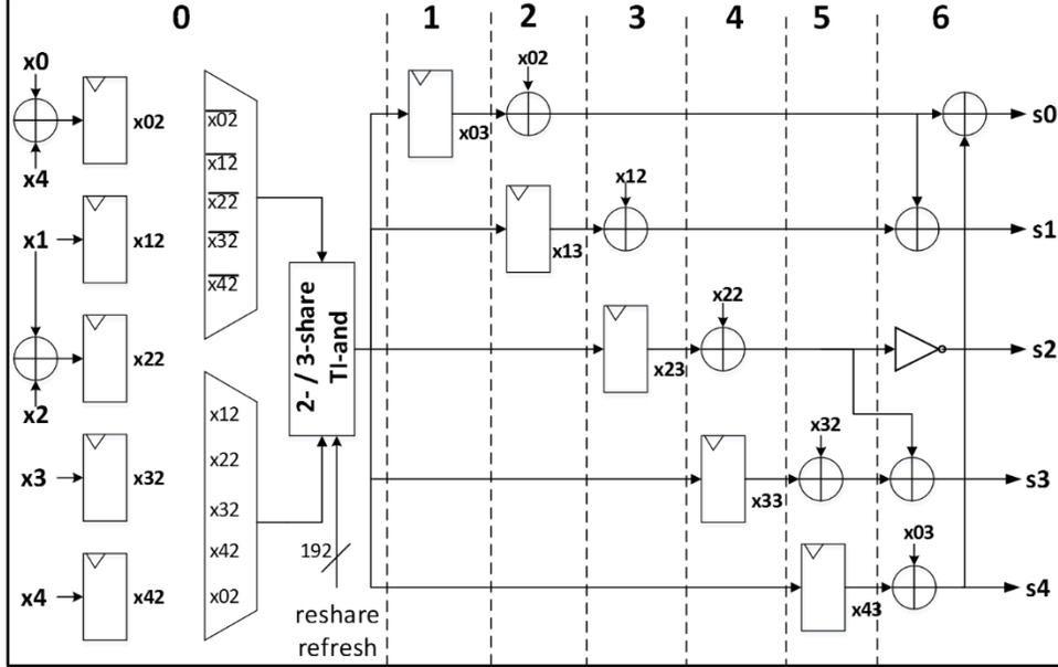
Fig. 6. 7-cycle ASCON S-Box. Stages are separated by dashed lines, and numbered across the top. All bus widths are 64-bits, unless indicated.
