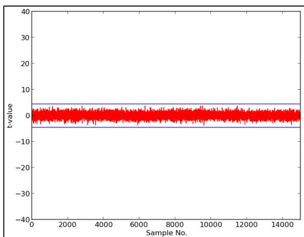
Fig. 15 Successful t-test of JAMBU-AES after modification of AEAD, including Pre- and Post-Processors.
