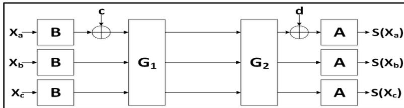
Fig. 10 3-share TI-protected S-Box used in authenticated ciphers with PRESENT and LED, adapted from [22, 42, 43]. A and B are matrix multiplications; c and d are constants; G is a quadratic composite function. All bus widths are 4 bits.
