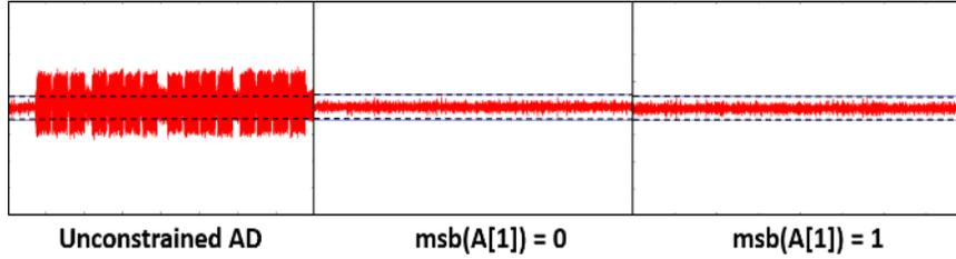
Fig. 19. Results of t-tests on protected implementation of CLOC-TWINE, with unconstrained test vectors on left, and test vectors  $AD_0$  and  $AD_1$  in center, and right, respectively. Time domain (samples) are on the x-axis, t-values are on the y-axis. The horizontal lines denote  $t = \pm 4.5$ .
