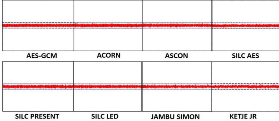
Fig.17. Results of t-test on AES-GCM, ACORN, ASCON, SILC, JAMBU (SIMON), and KETJE authenticated ciphers, protected against 1<sup>st</sup> order DPA. The dashed lines denote  $t = \pm 4.5$ .
