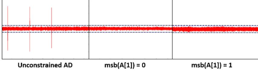
Fig. 18. Results of t-tests on protected implementation of CLOC-AES, with unconstrained test vectors on left, and test vectors  $AD_0$  and  $AD_1$  in center, and right, respectively. Time domain (samples) are on the x-axis, t-values are on the y-axis. The horizontal lines denote  $t = \pm 4.5$ .
