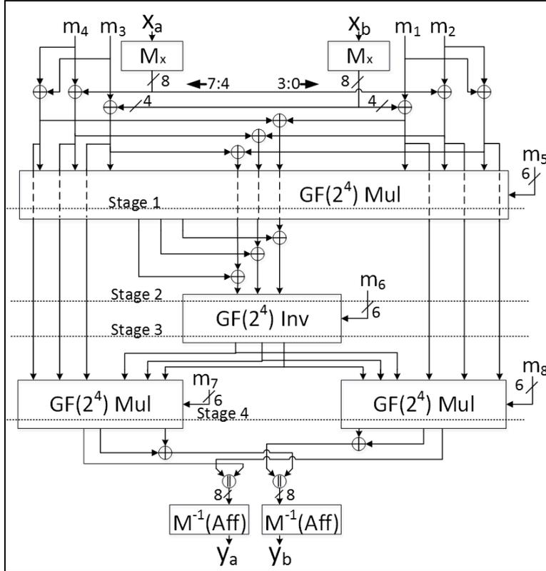
Fig. 7. 8-bit 5-stage pipelined TI-protected S-Box. Dotted lines denote stage boundaries; dashed lines indicate pass-thru, i.e., no interaction with component.  $M_x$  represent change to normal basis, and  $M^{-1}$  are combined affine transformation and change to standard basis.  $m_i$  indicate random refresh bits, with bus widths as indicated. Adapted from [22].
