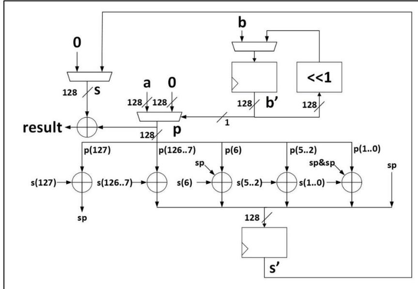
Fig. 8. 3-share TI-protected  $GF(2^{128})$  multiplier used in AES-GCM. All signals are triplicated inside the multiplier for three-share computation.
