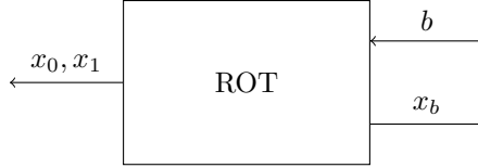
Figure 2: Random Oblivious Transfer. In the ROT functionality, the sender provides no input to the protocol, and instead the values x_0, x_1 are generated uniformly at random by the protocol itself.
