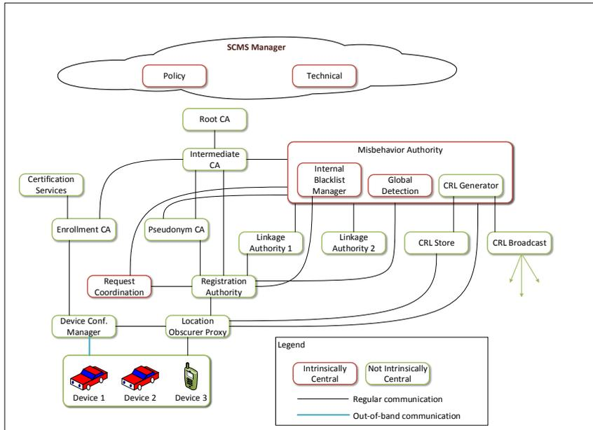
**Figure 1:** Overview of SCMS's architecture. Source:[12].
