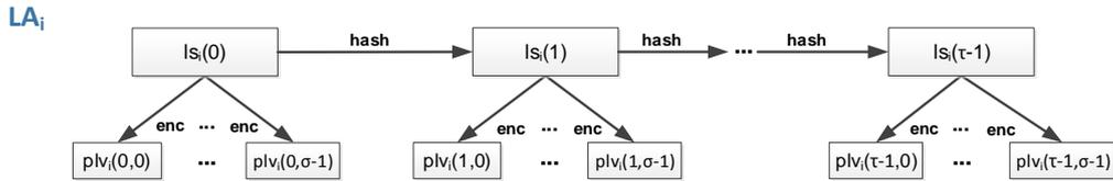
**Figure 3:** SCMS's key linkage tree:  $LA_i$  generates the linkage seeds ( $ls$ ) and pre-linkage values ( $plv$ ) employed for certificate revocation/linkage.
