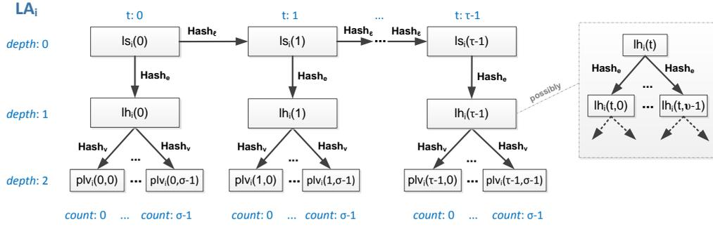
**Figure 4:** Proposed certificate linkage tree: adding linkage hooks and security strings.
