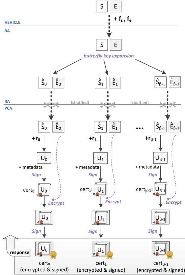
**Figure 2:** SCMS's butterfly key expansion and certificate generation.
