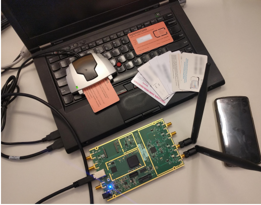
Fig. 4. Our experimental setup, showing a smartcard reader, USRP (left), set of commercial USIM cards, and a test phone.
