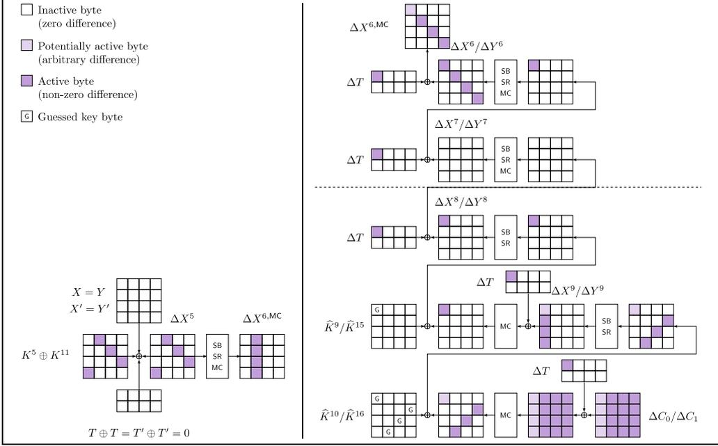
**Figure 4:** Trails of our ten-round rectangle attack. **Left:** Top trail over Round 6. **Right:** Bottom trail, covering the round-key and tweak addition in Round 6 and Rounds 7 through 10. The operations below the dashed horizontal line are considered during the key recovery.
