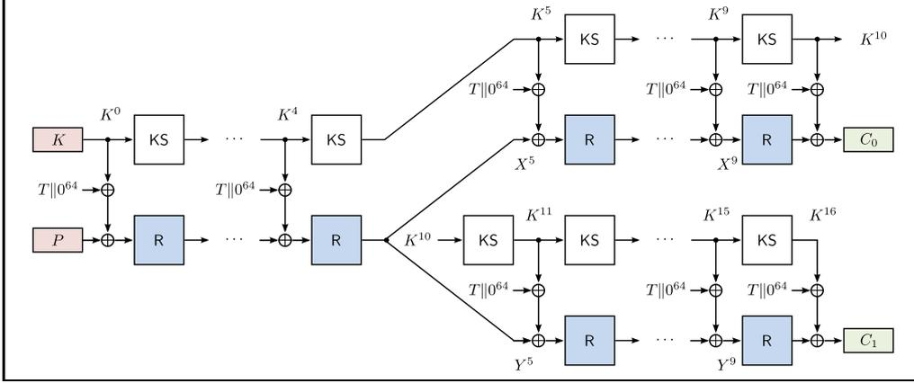
**Figure 1:** ForkAES. R denotes the round function and KS an iteration of the AES-128 key schedule.
