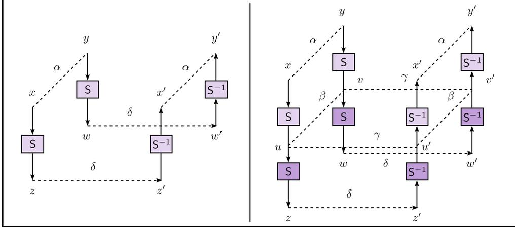
**Figure 5: Left:** The setting of Cid et al.’s Boomerang-connectivity Table; **Right:** Our setting for verifying the middle phase, where  $\alpha = X^5[9] \oplus Y^5[9]$ ,  $\gamma = \Delta X^6[5]$ , and  $\delta = \Delta X^{7,SR}[1]$ .
