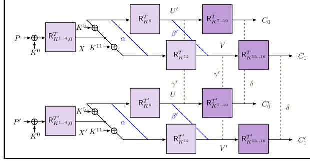
**Figure 3:** Schematic illustration of our weak-key rectangle attack on ten-round ForkAES.
