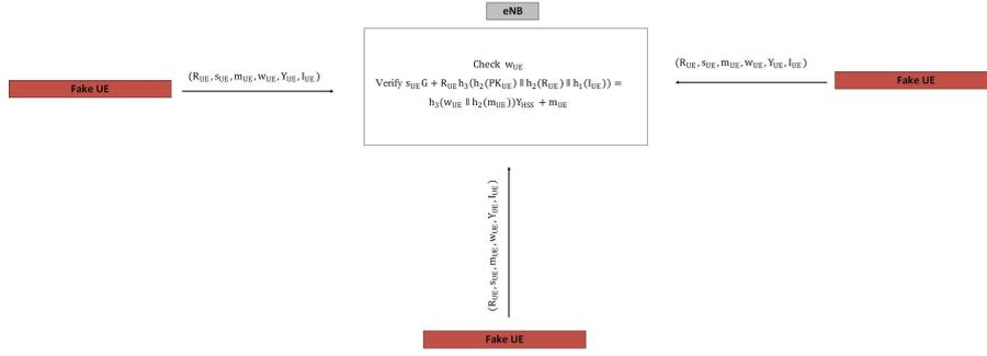
**Fig. 2** DoS attack against Qui et al.'s handover scheme
