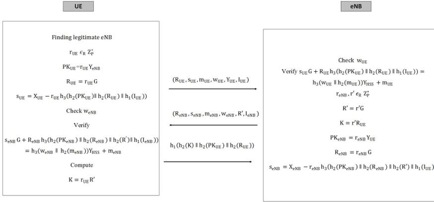
**Fig. 1** Normal handover phase of the Qui et al.'s scheme
