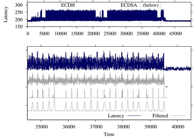
Figure 6. Multiple TLS trace stages. Top: Raw TLS handshake trace showing scalar multiplication during ECDH and ECDSA. Bottom: Zoom at the end of the previous ECDSA trace, peaks (filtered) represent Add operations. For example, this trace ends with an add operation, indicating the nonce is odd.
