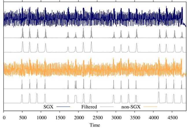
Figure 8. From top to bottom: raw trace of our SGX Victim; said trace after filtering; raw trace of our user space Victim; said trace after filtering. Both victims received the same input, i.e. a scalar that induces 16 point additions at the end of the trace, clearly identifiable by the peaks in the filtered traces. This demonstrates the leakage from SGX is essentially identically to the leakage outside SGX.
