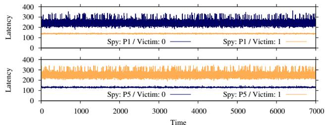
Figure 5. Top: Timings for the PORTSMASH Spy when configured with P1, in parallel to the Victim executing `x64_foo` with `rdi` as both zero and one in two consecutive runs. Bottom: Analogous but with the Spy configured with P5.
