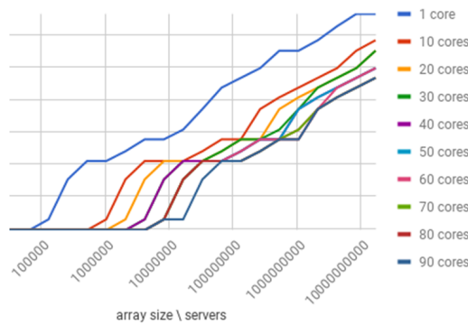
Figure 3: Running time ( y -axis) of our system using multiple machines (in color) on the cloud for different number of database records ( x -axis). As implied by the analysis, the running time reduces linearly with number of machines, unlike existing secure implementations or the direct method that do not use coresets.
