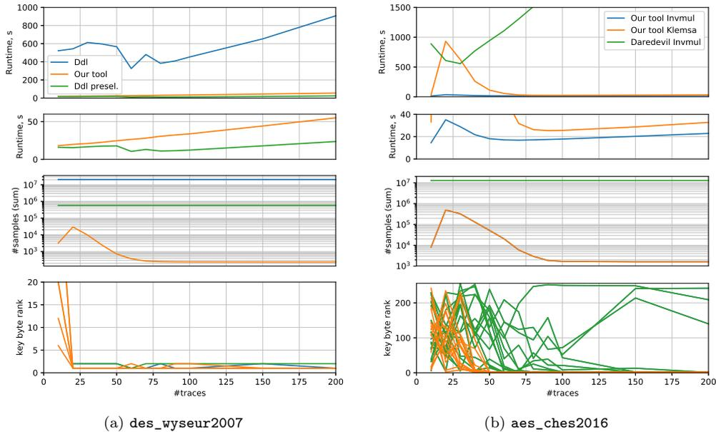
Figure 2: Different attack metrics vs number of traces. Top to bottom: runtime; zoomed-in runtime; total number of samples going into correlation computation; correct key chunk candidate ranks.
