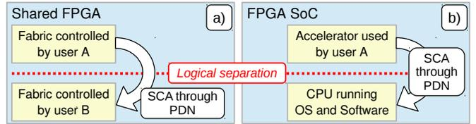
Fig. 1: Two scenarios of SCA attacks, where the circuits are logically separated, but share the same PDN. **a)** In a shared FPGA, one user (A) can attack another (B). **b)** In an FPGA SoC, a user with current access to the FPGA accelerator can attack any software or operating system on the CPU.
