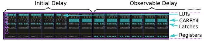
Fig. 3: Floorplan (rotated right) of one TDC Sensor with  $18 \times (\text{LUT}, \text{Latch})$  as part of the Initial Delay.
