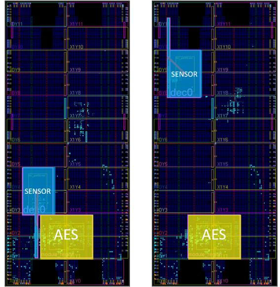
Fig. 6: Floorplans showing the Experimental Setup with all the relevant parts. **Left:** the internal sensor is placed close to the AES module. **Right:** the internal sensor is placed far away from the AES.
