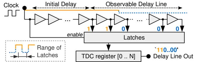
Fig. 2: Principle of the TDC Sensor from [10].
