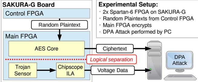
Fig. 5: Experimental setup showing the Sakura-G Board connected to our measurement PC, with Chipscope ILA used for data acquisition.
