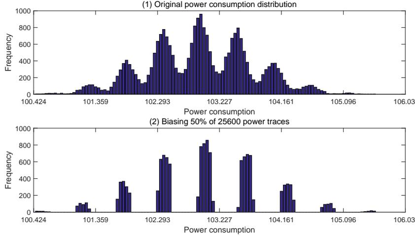
**Figure 3:** Biasing power traces using our TLOB.
