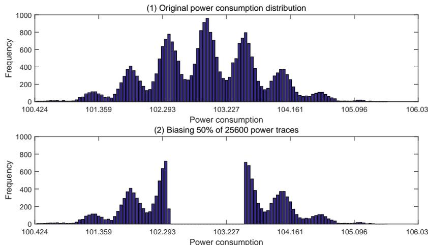
**Figure 1:** Using DTOB to bias 50% of 25600 power traces.
