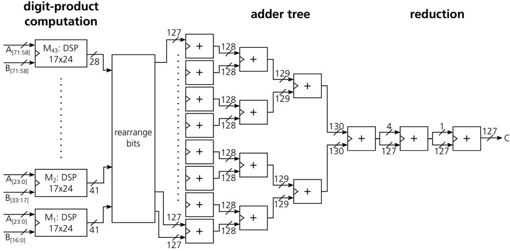
**Figure 3:** Architecture of the  $127 \times 127$ -bit multiplier modulo  $2^{127} - 1$ .
