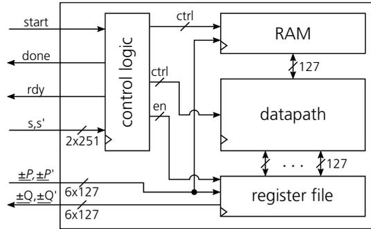
**Figure 1:** Single-core architecture, which contains all control and datapath logic for computing Algorithm 1 (`scalar_mult`).
