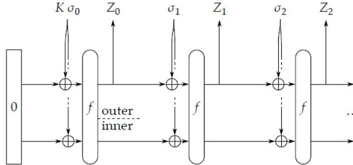
Fig. 3. The full-state keyed duplex construction applied in Keyak [BDP<sup>+</sup>e]
