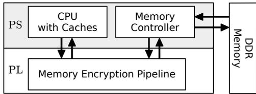
Fig. 1. Zynq platform with memory encryption module.
