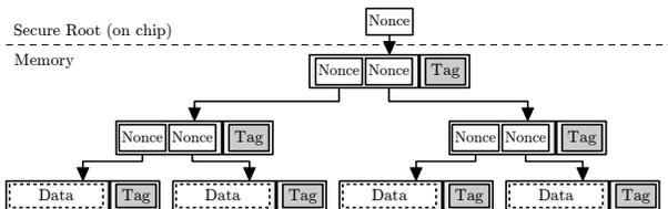
Fig. 4. Binary Tamper Evident Counter (TEC) tree.
