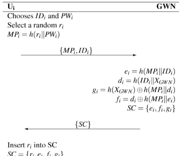
**Figure 1. User Registration phase of Farash et al.'s scheme [8].**
