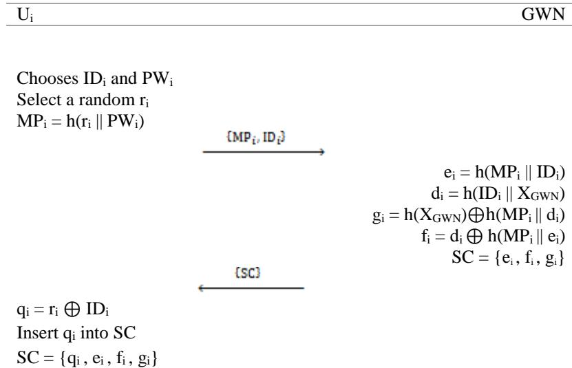
**Figure 4. User registration phase of the proposed scheme.**
