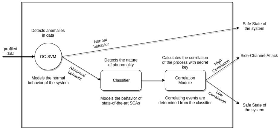
Fig. 3: Basic overview of the detection mechanism
