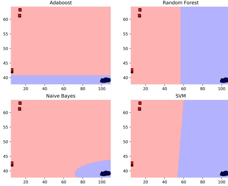
Fig. 5: Decision Boundary of different Classifiers on some of the side-channel-attacks
