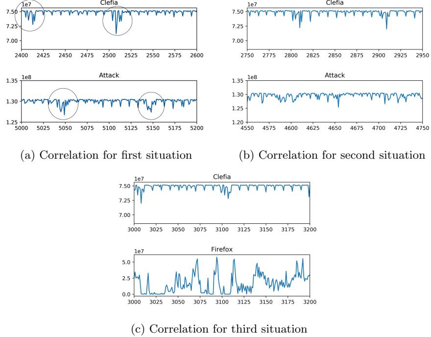
Fig. 6: Correlation with key for different situations
