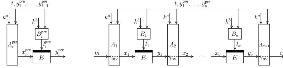
Fig. 3: Tweakable blockcipher  $\tilde{E}[\rho, \sigma]$ : precomputation of  $y_i^{\text{pre}}$  (left) and processing of  $m$  (right). “inv.” means that the function is invertible
