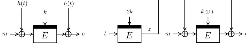
Fig. 1: Tweakable blockcipher LRW2      Fig. 2: Tweakable blockcipher Men2
