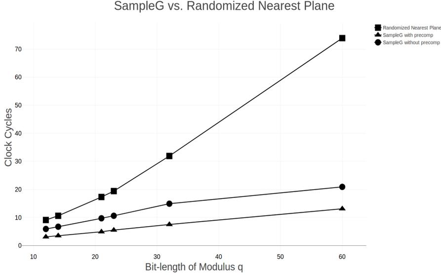
Figure 3: Measured clock cycles with  $q = \{4093, 12289, 1676083, 8383498, 4295967357, \approx 9 \cdot 10^{18}\}$  and  $s = 100$  averaged over 100,000 runs. The clock cycles for the last three moduli are  $\{19.4, 31.9, 73.9\}$  for GPV and  $\{5.5, 7.5, 13.1\}$  for SAMPLEG with pre-computation.
