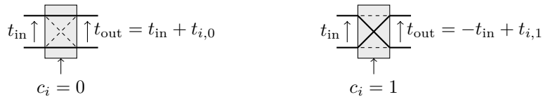
Figure 2: The delay behavior of a single stage of an Arbiter PUF. If for a given challenge \mathbf{c} , the delay difference between the upper and lower path accumulated to t_{\text{in}} after the first i - 1 stages, then stage i adds either t_{i,0} or t_{i,1} , depending on the value of challenge bit c_i . Note that for c_i = 1 , the upper and lower paths are reversed, and the sign of t_{\text{in}} is flipped accordingly.
