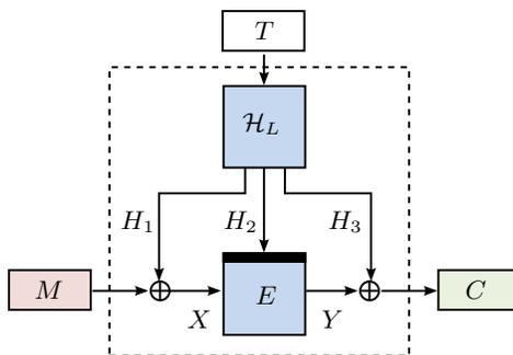
**Fig. 1:** Schematic illustration of the encryption process of a message  $M$  and a tweak  $T$  with the general  $\text{GXHX}[E, \mathcal{H}]$  tweakable block cipher.  $E : \mathcal{K} \times \{0, 1\}^n \rightarrow \{0, 1\}^n$  is a keyed permutation and  $\mathcal{H} : \mathcal{L} \times \mathcal{T} \rightarrow \{0, 1\}^n \times \mathcal{K} \times \{0, 1\}^n$  a keyed universal hash function.
