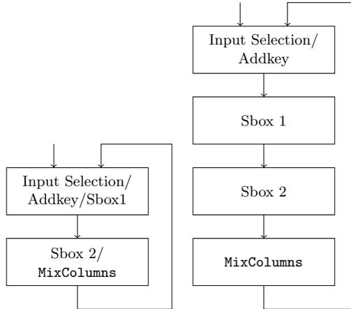
Fig. 9: Two/Four-Stream AES round data path implementation
