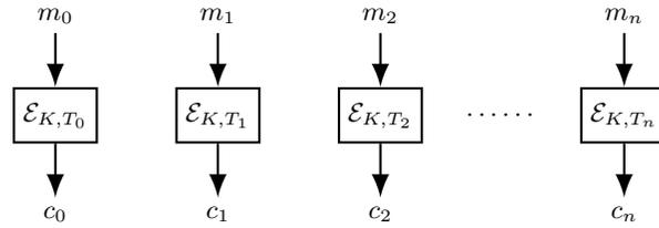
Fig. 2: The parallel encryption structure
