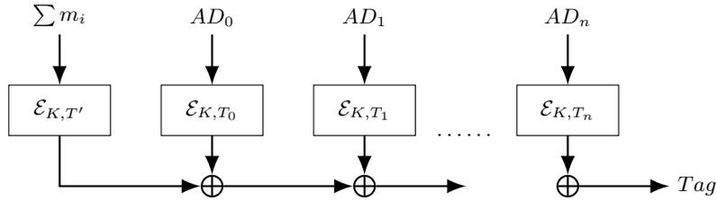
Fig. 3: The encrypt-then-xor construction
