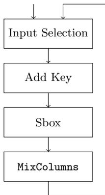
Fig. 5: The AES encryption data path from [14]
