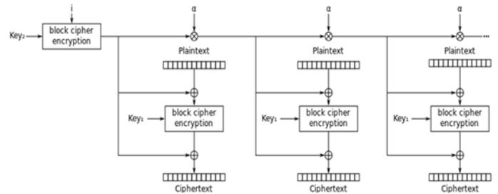
Figure 3. XTS Encryption Mode
