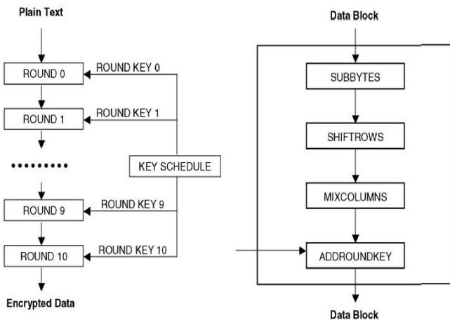
Figure 4. Iterative cipher with key schedule
