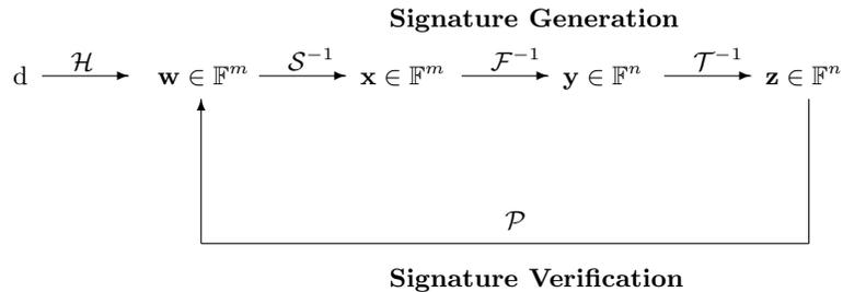
**Fig. 2.** General workflow of multivariate signature schemes
