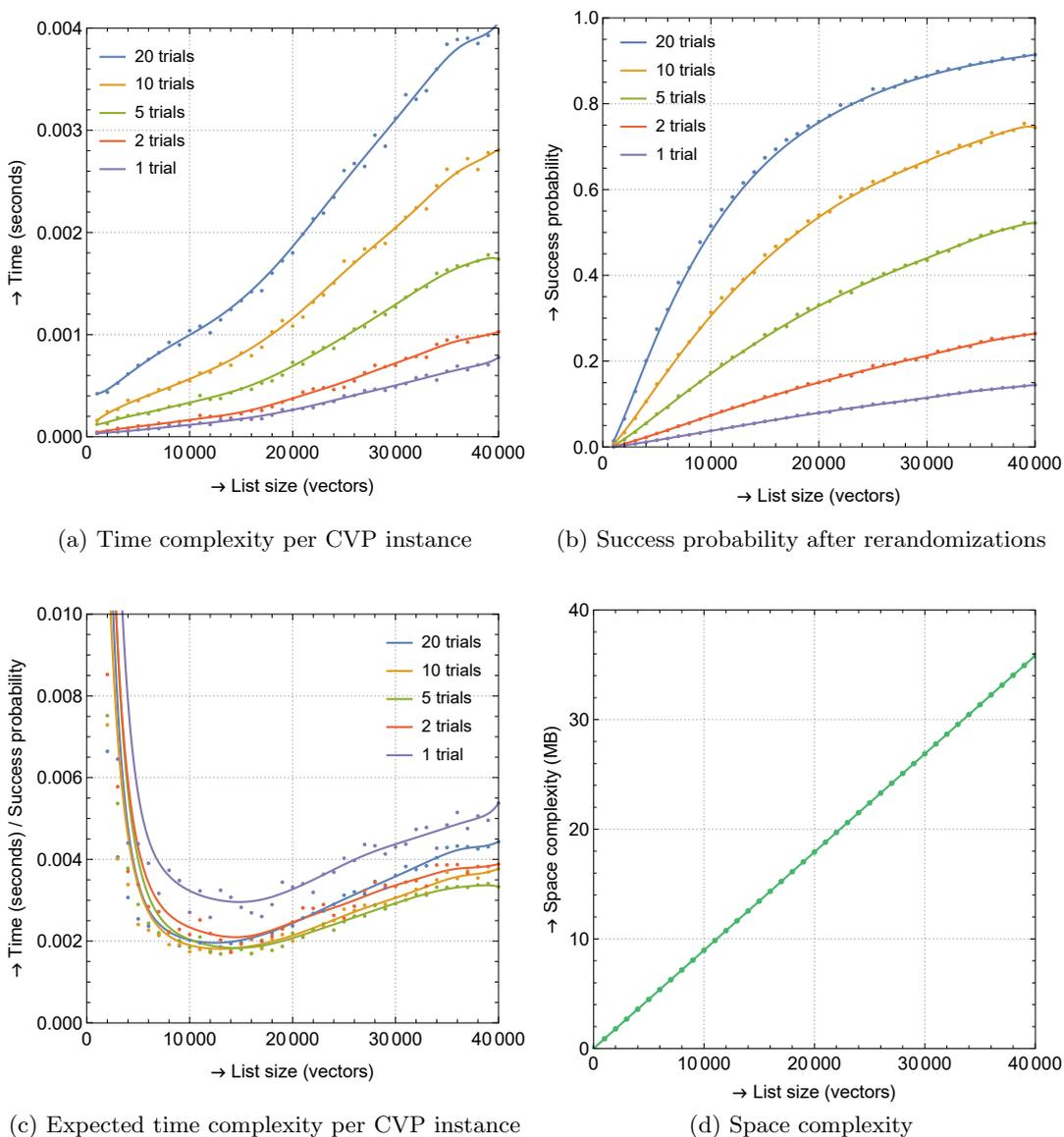
**Fig. 6.** Experimental results for solving CVPP with randomized sieving. Figure 6a displays the average time complexity per instance. Figure 6b shows the average success probability after rerandomizations. Figure 6c displays expected time costs, taking into account the success probability. Figure 6d displays the space complexity of the data set and the indexed data structure. Each data point corresponds to 10 000 random target vectors for this choice of parameters.
