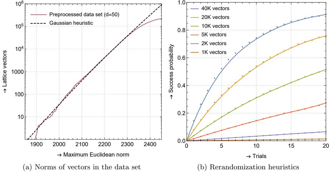
**Fig. 5.** Verifying the heuristic assumptions. Figure 5a compares the norms of the vectors in the data set to the expected norms of the shortest vectors in the lattice, based on the Gaussian heuristic. Figure 5b depicts how rerandomizations affect the success probability. Different curves in Figure 5b correspond to a different number of preprocessed vectors being used for reductions.
