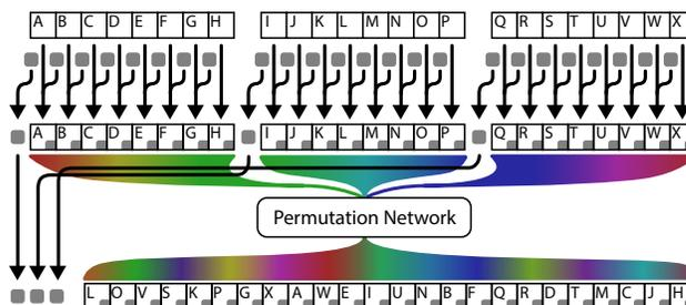
(b) **Interleaving multiple arrays to form an oblivious linked multi-list.** Multiple arrays can be concatenated and permuted together, becoming indistinguishable from one another. Individual entry points allow them to be independently traversable.
