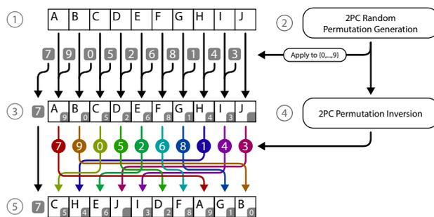
(a) **Initialization.** The input ① is combined with a random permutation ② which has been shifted left by one place. The result ③ is then permuted according to the inverse of the first permutation ④, resulting in a shuffled linked list ⑤. The leftmost element of the first random permutation ② is retained outside the structure and represents the entry point.
