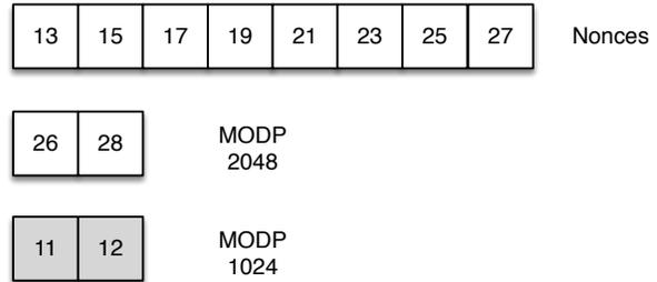
**Figure 2:** Queue state after 8 MODP 2048 exchanges. Numbers indicate generation order, and stale values are highlighted. If several connections have been made to the same DH group, the other DH group can grow stale as all nonces that were generated before those keys are used up.
