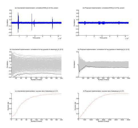
Fig. 4: Side-channel power analysis results: the left side are the results of attacking the original implementation, the right side are the results of attacking the implementation protected with the proposed scheme.
