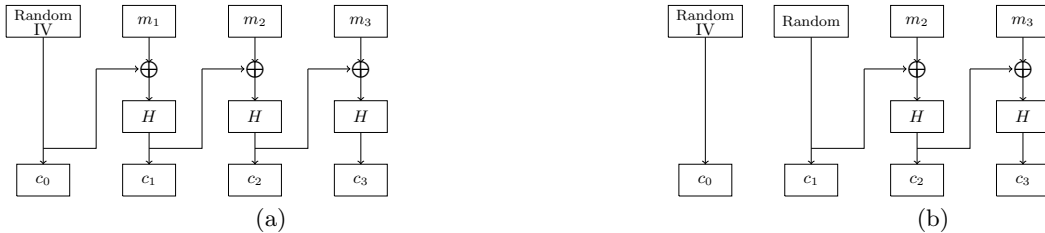
Fig. 1: (a) CBC mode (using a random function H instead of the block cipher). (b) Modified challenge ciphertext computation ( c_1 replaced by randomness). We need to prove that replacing c_2 by a random value leads to an indistinguishable view.
