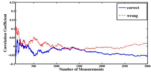
Fig. 2. Number of measurements vs. Correlation Coefficient targeting  $64^{th}$  key bit using **random** IVs.
