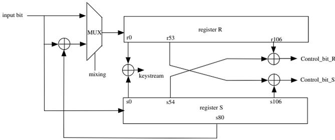
Fig. 1. Hardware realization of MICKEY-128 2.0 stream cipher.
