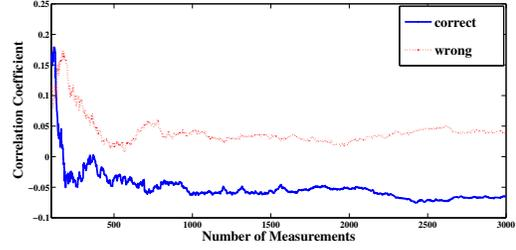
Fig. 3. Number of measurements vs. Correlation Coefficient targeting 64<sup>th</sup> key bit using PSO generated IVs.
