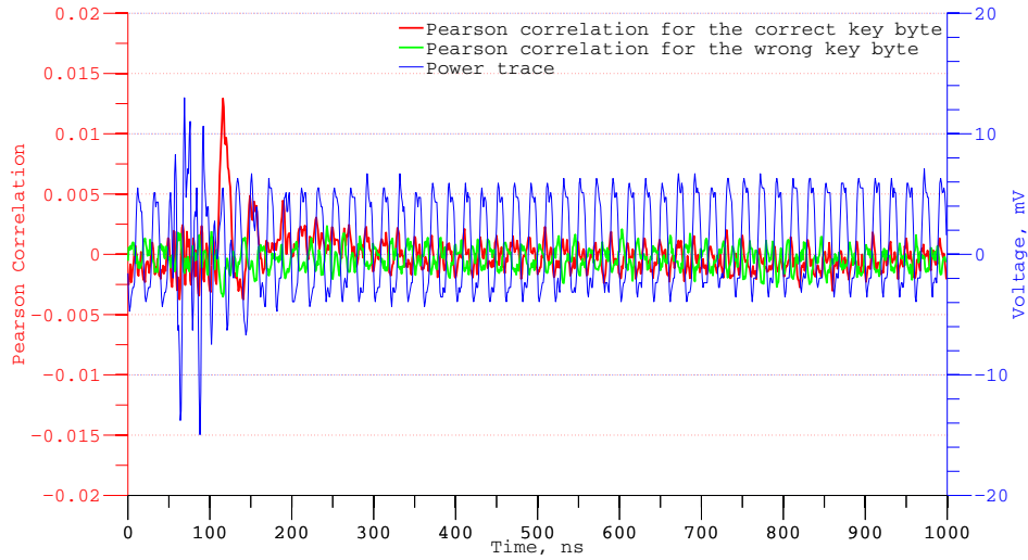
Fig. 4. Unprotected implementation: Pearson correlation value of a correct (red) and an incorrect (green) key byte guess. 500,000 power traces.
