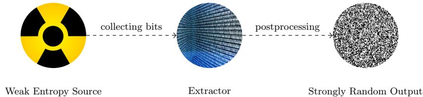
Fig. 1: True Random Number Generators. The scheme illustrates the typical design, where the building blocks are: (a) an entropy source (b) a harvesting mechanism and (c) a postprocessor (extractor).
