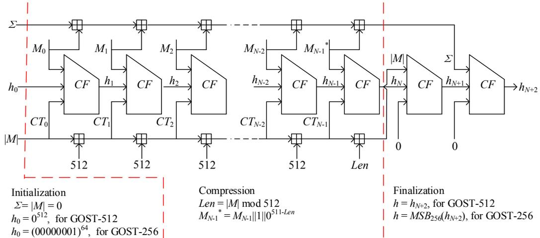
**Fig. 1.** Three stages of the GOST hash function
