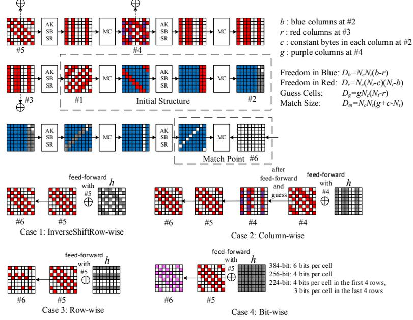
Fig. 8. MitM preimage attack on 6-round AES-like compression function
