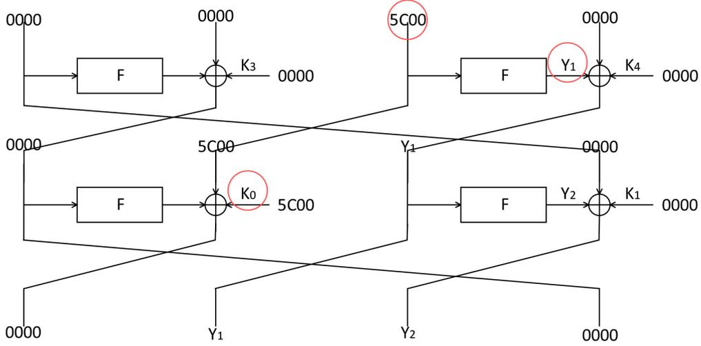
Fig. 3: The differential propagation pattern of  $E_f$
