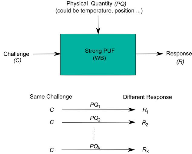
**Fig. 1.** Response (R) of the PUF is a function of the Challenge (C) and Physical Quantity (PQ). For the same C, different R are produced due to the difference of PQ.
