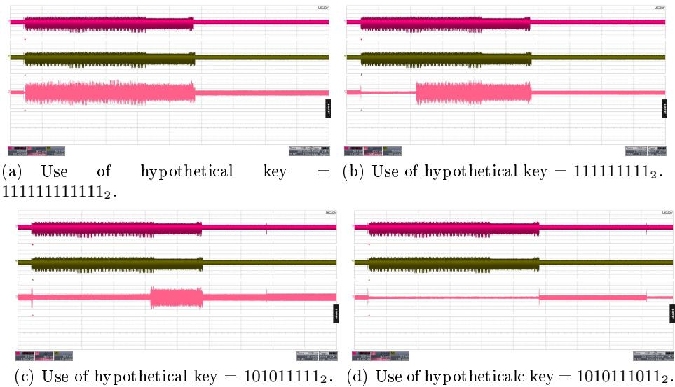
**Fig. 7.** Exemplary Results of the classification ‘wd’ using the sliding window exponentiation on elliptic curve secp160r1 and projective coordinates. In each figure, the top curve is the single measurement of the guessed scalar and the second curve is the single measurement of the secret scalar. If the bit sequences are made more equal, the differences approaches zero in the third curve.
