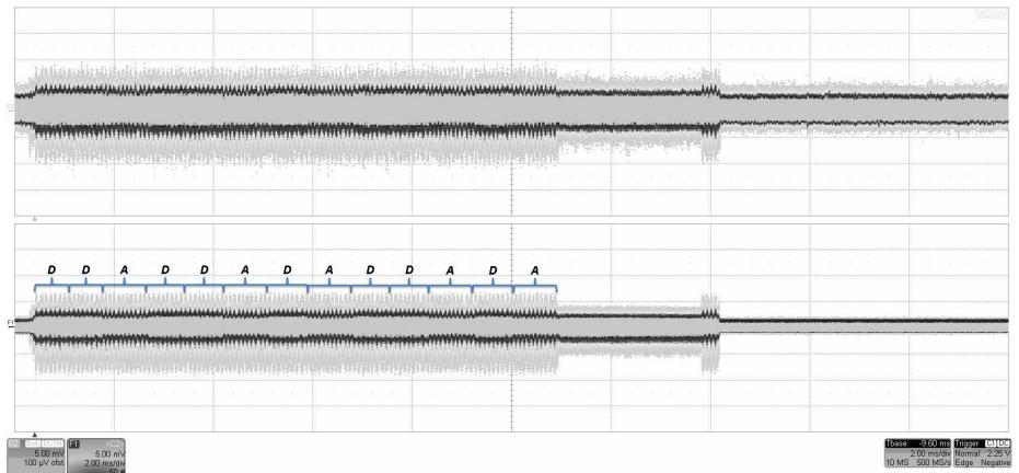
(b) Classification 'a': Configuration "Curve-Specific Optimization" using projective co-ordinates and secp192r1 elliptic curve parameter.
