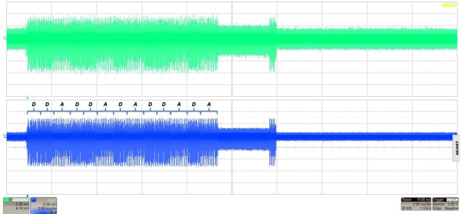
(a) Classification 'a': Configuration "Curve-Specific Optimization" using projective co-ordinates and secp160k1 elliptic curve parameter.
