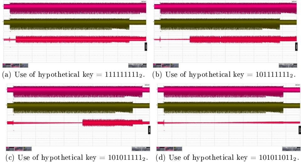
**Fig. 5.** Exemplary Results of the classification 'd' using secp128r1 elliptic curve parameter. In each figure, the top curve is the single measurement of the guessed scalar and the second curve is the single of the secret scalar. If the bit sequences are made more equal, the differences approaches zero in the third curve.
