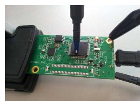
(c) LF-U-2,5 positioned on the surface of the microcontroller.
