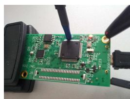
(b) LF-B-3 positioned near the VCC pin.
