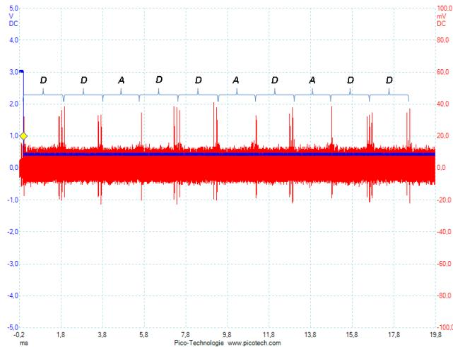
(b) Classification 's-': Configuration "Curve-Specific Optimization" with affine coordinates and the secp128r1 elliptic curve parameter.
