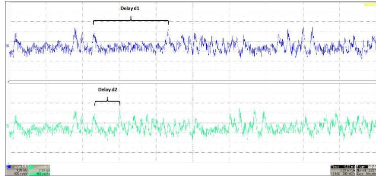
**Fig. 6.** Delay caused by the bit length of the scalar.
