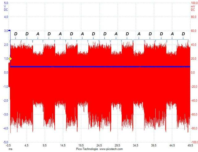
(a) Classification 's+': Configuration "Simply" with affine coordinates and the secp160r1 elliptic curve parameter.
